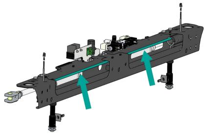
Figure 13: Spiral cable guiding shaft
