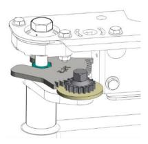
Figure 15: torque tool VA3860
